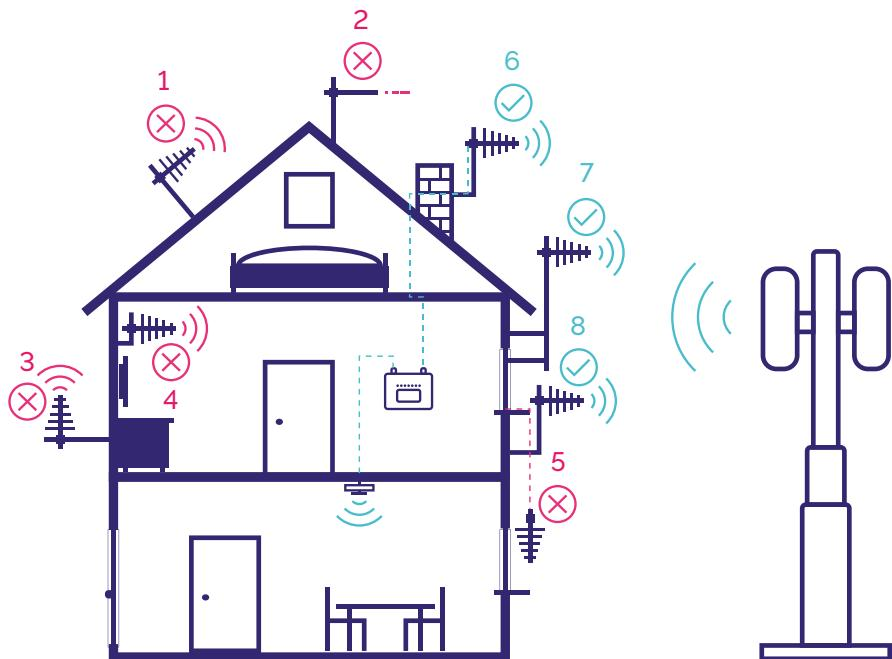
1. Do not install the antenna on the roof slope.
